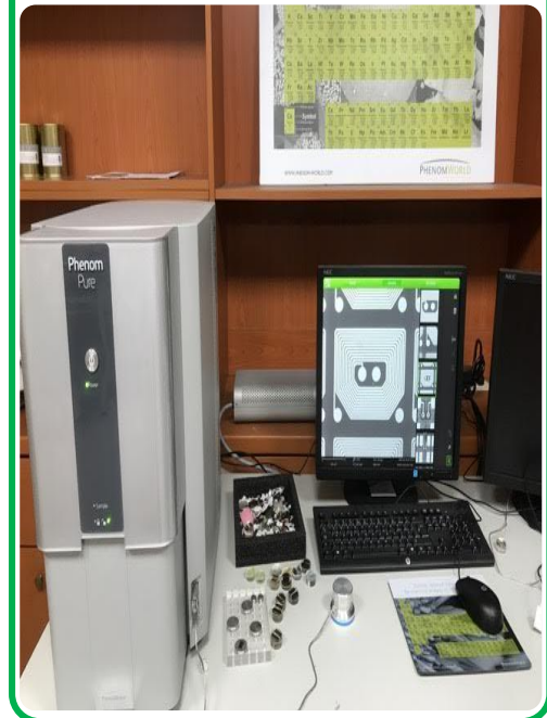
Scanning electronic microscope (For material analysis)
