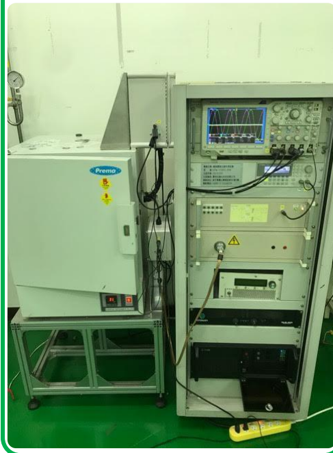
High frequency B-H analyzer (core loss measurement)
